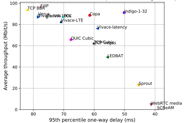
test from Mexico Ethernet to AWS California 2 Ethernet, 10 runs of 30s each per scheme
