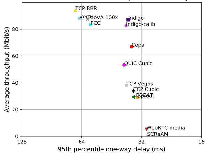
test from Mexico Ethernet to AWS California 2 Ethernet, 10 runs of 30s each per scheme
