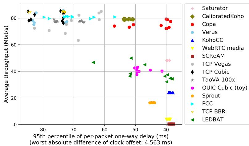
test from Mexico Ethernet to AWS California 2 Ethernet, 10 runs of 30s each per scheme
