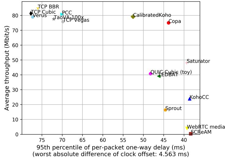
test from Mexico Ethernet to AWS California 2 Ethernet, 10 runs of 30s each per scheme
