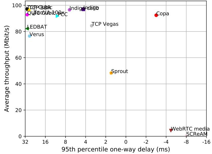
test from AWS India 1 Ethernet to India Ethernet, 10 runs of 30s each per scheme
