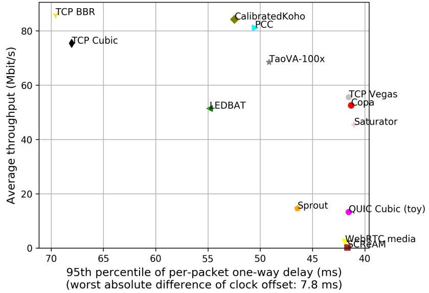
test from AWS India 1 Ethernet to India Ethernet, run 1 of 30s each per scheme
