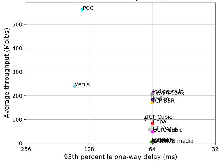
test from GCE Tokyo Ethernet to GCE Iowa Ethernet, 10 runs of 30s each per scheme
