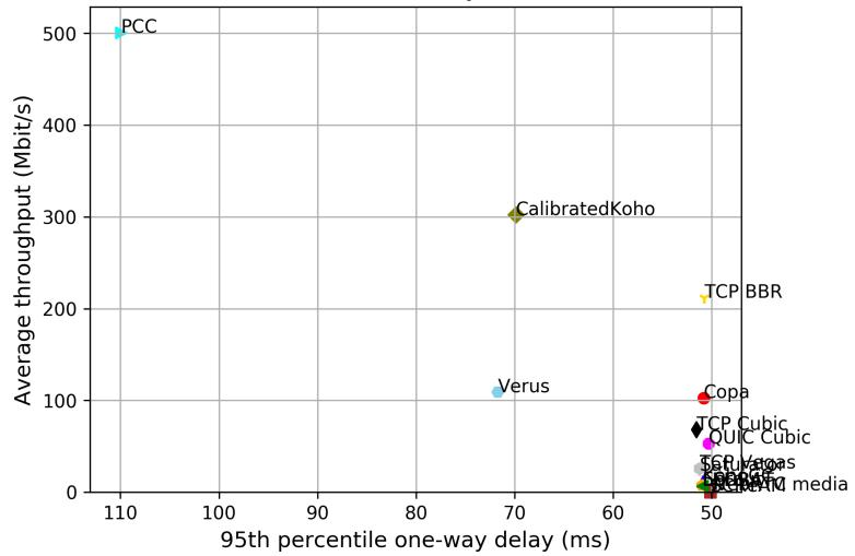
test from GCE London Ethernet to GCE Iowa Ethernet, 10 runs of 30s each per scheme
