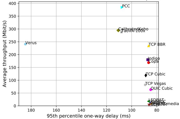
test from Colombia Ethernet to AWS Brazil 2 Ethernet, 10 runs of 30s each per scheme
