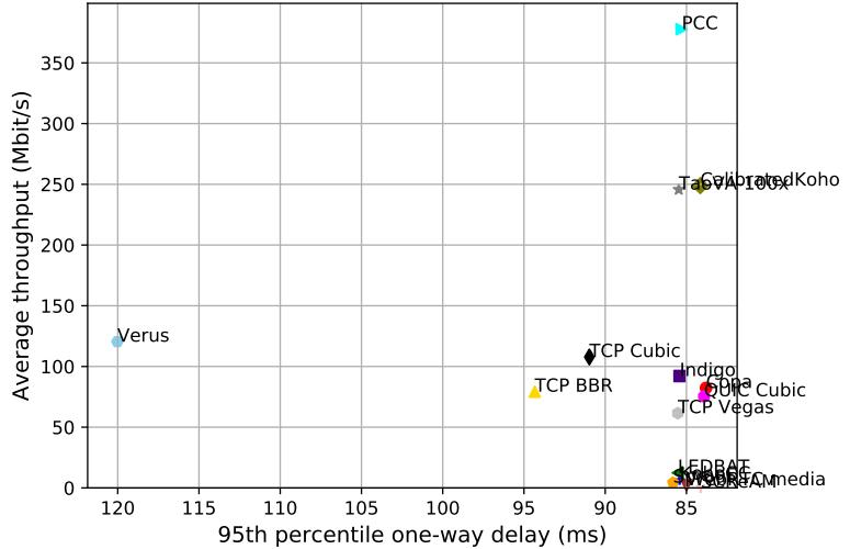
test from AWS Brazil 2 Ethernet to Colombia Ethernet, 10 runs of 30s each per scheme
