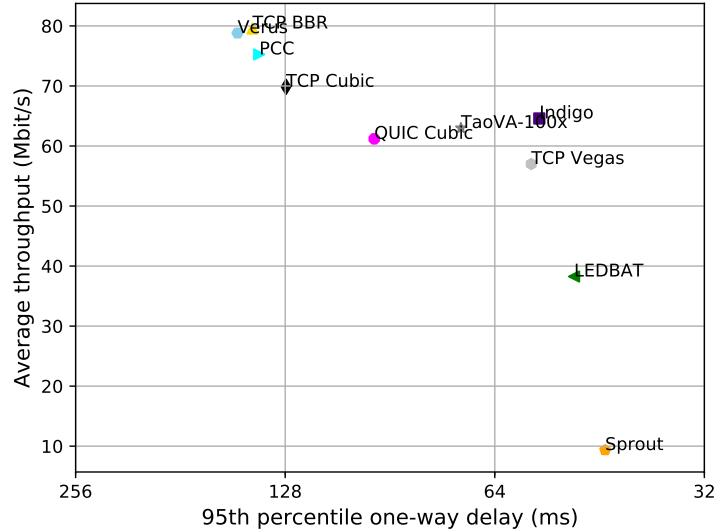
test from China Ethernet to AWS Korea Ethernet, 10 runs of 30s each per scheme
