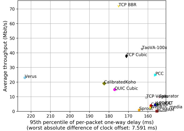
test from China Ethernet to AWS Korea Ethernet, 10 runs of 30s each per scheme
