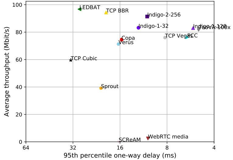
test from AWS Brazil 1 Ethernet to Brazil Ethernet, 10 runs of 30s each per scheme
