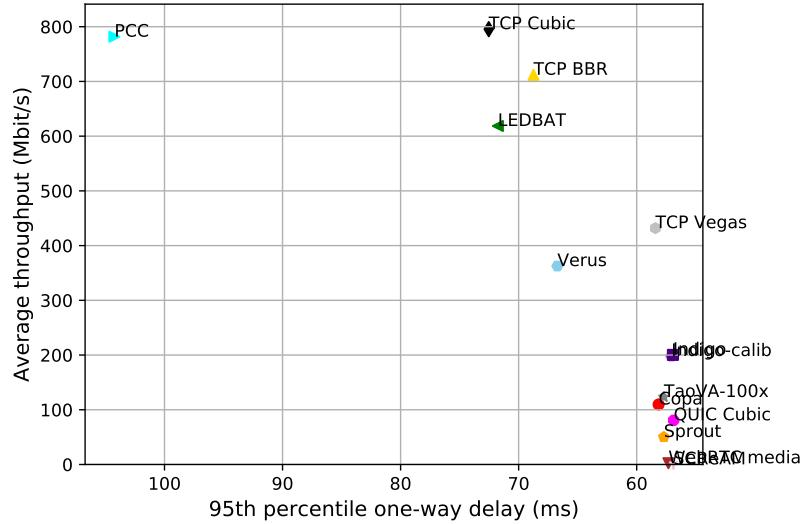
test from AWS Brazil 1 Ethernet to Brazil Ethernet, 10 runs of 30s each per scheme
