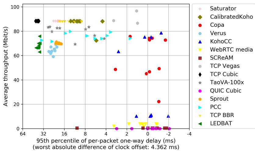
test from AWS Brazil 1 Ethernet to Brazil Ethernet, 10 runs of 30s each per scheme
