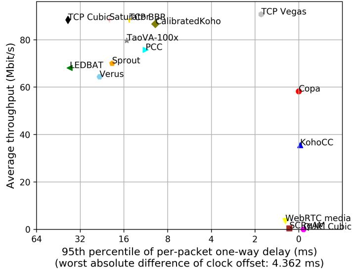
test from AWS Brazil 1 Ethernet to Brazil Ethernet, 10 runs of 30s each per scheme
