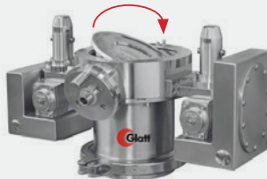
2. Turning the valve disc by 180 degrees.
