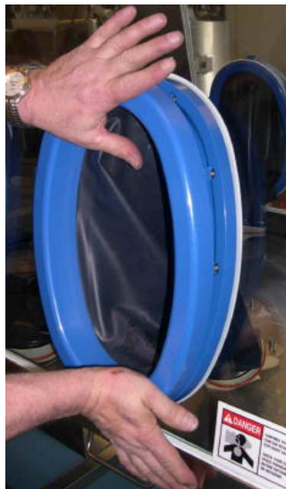
Align the retainer with the gloveport and start the retainer with a gentle rocking top and bottom motion.
