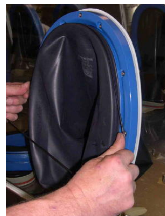
Start the glove sleeve attachment o-ring in the outer groove over the sleeve.
