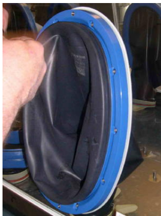
Check to see that the sleeve bead is firmly seated in the inner groove and there are no twists or folds in the sleeve as it forms to the edge of the port.
