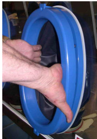
Seat the retainer by pulling the retainer and port together with a clamping motion of your hands as shown above.
