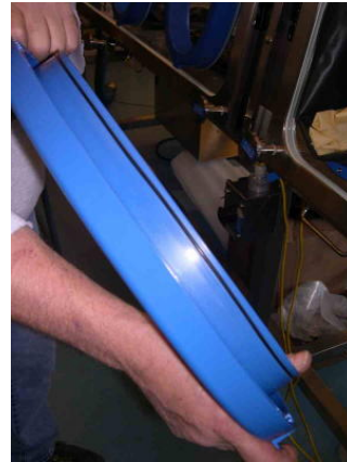
Check the retainer to verify the retainer o-ring is installed in the retainer groove
