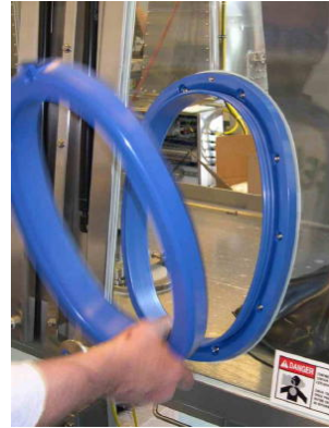
Remove the retainer from the gloveport assembly.
