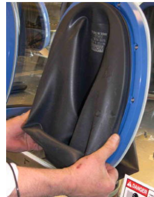
Continue the installation by stretching the glove bead to fit the port – Note: be certain that you are installing the correct glove (i.e. 10" glove for a 10" port).
