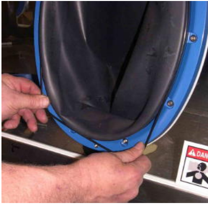
Stretch the o-ring to fit and insure it is seated in the outer groove of the port
