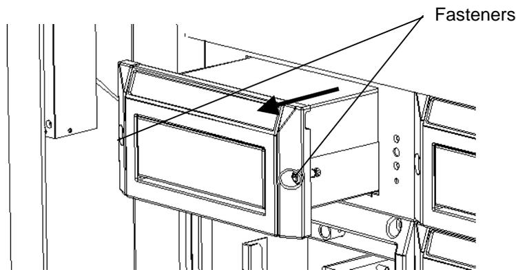
Figure 33. Fasteners on the Incubator Modules or Detection Module
