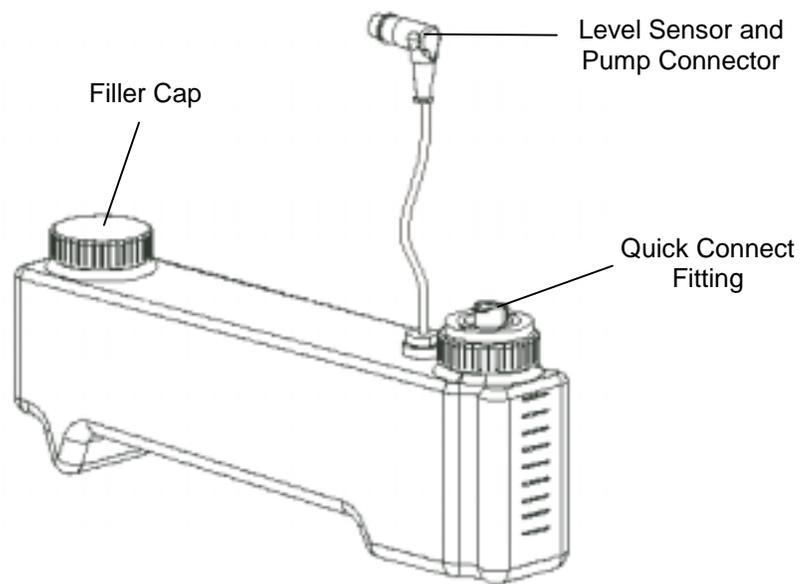
Figure 12. Wash Buffer Container Details
