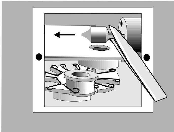
Figure 35. Removing the Lamp
