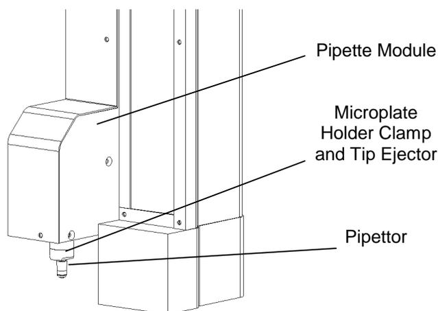
Figure 7. The Pipette Module
