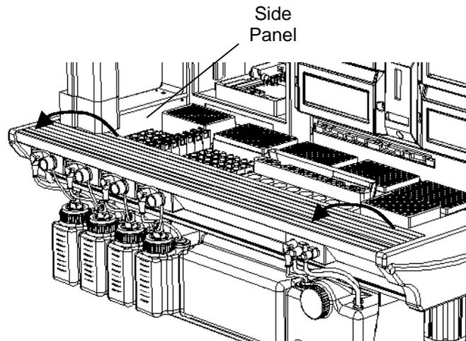
Figure 37. Lifting the Front Panel
