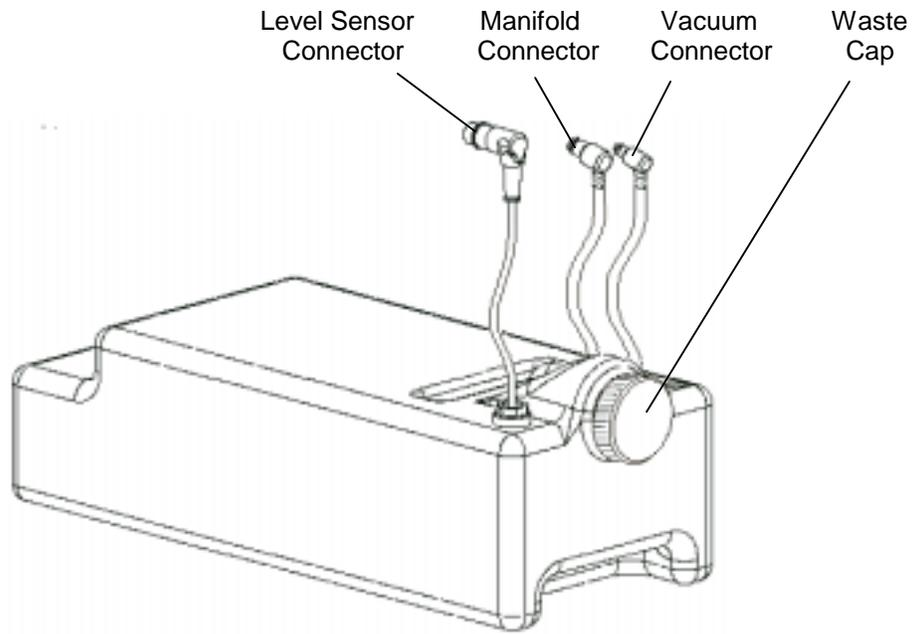
Figure 14. Liquid Waste Container
