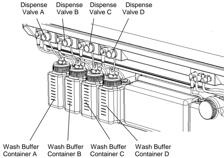
Figure 11. Wash Buffer Containers and Wash Buffer Dispense Valves
