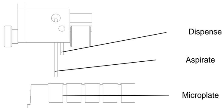
Figure 10. Position of the Wash Pins
