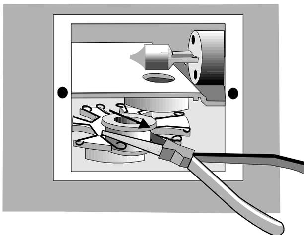
Figure 36. Removing a Filter
