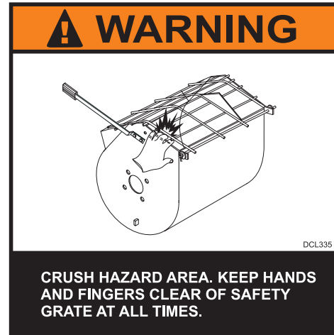
Figure 38. Safety Grate (Crush Hazard)
