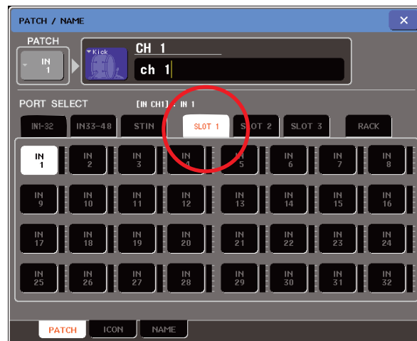
The Patch screen allows channels from the external MY card slots to be assigned to the M7CL faders.
