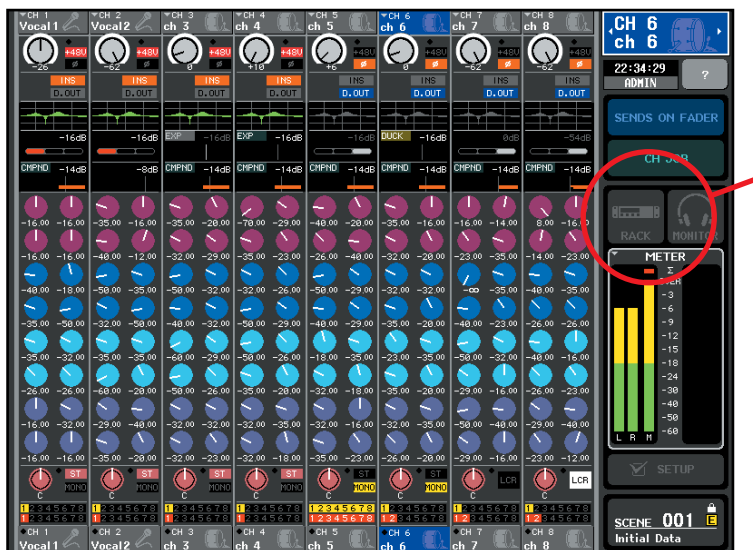
The M7CL touchscreen—the circle highlights the button used to access the Virtual Rack screen.
