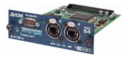
The 6416Y2 A-Net® Interface Card is a 16-channel input/output expansion card for Yamaha® products supporting Yamaha's mini-YGDAI (MY) format. Compatible products include most Yamaha digital mixing consoles, as well as Digital Mix Engine devices. The 6416Y2 A-Net card is compatible with all Aviom Pro64® Series products and, with an ASI A-Net Systems Interface module, can also be used with Pro16® Series output products, such as the industry standard A-16II Personal Mixer.
