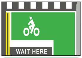
Bike boxes at intersections provide a space for bicyclists to stop in front of cars. This increases safety for bicyclists turning left because they can wait ahead of vehicles at a red light and are more visible to drivers.
