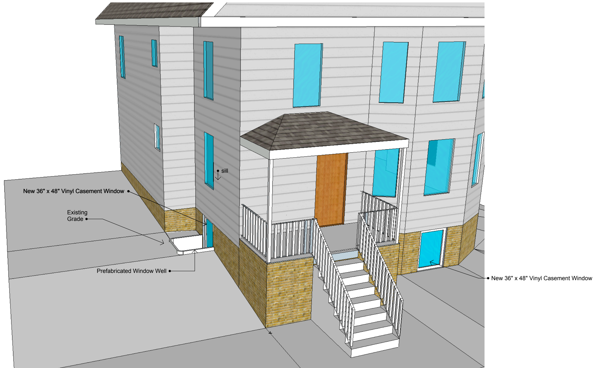
Elevation A Showing New Basement Windows
