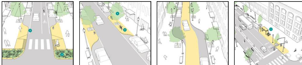
Figure 25. Curb extension design options highlighted in yellow, including (from top left to bottom right): Gateway, Pinchpoint, Chicane, and Bus Bulb. (NACTO 2013).
