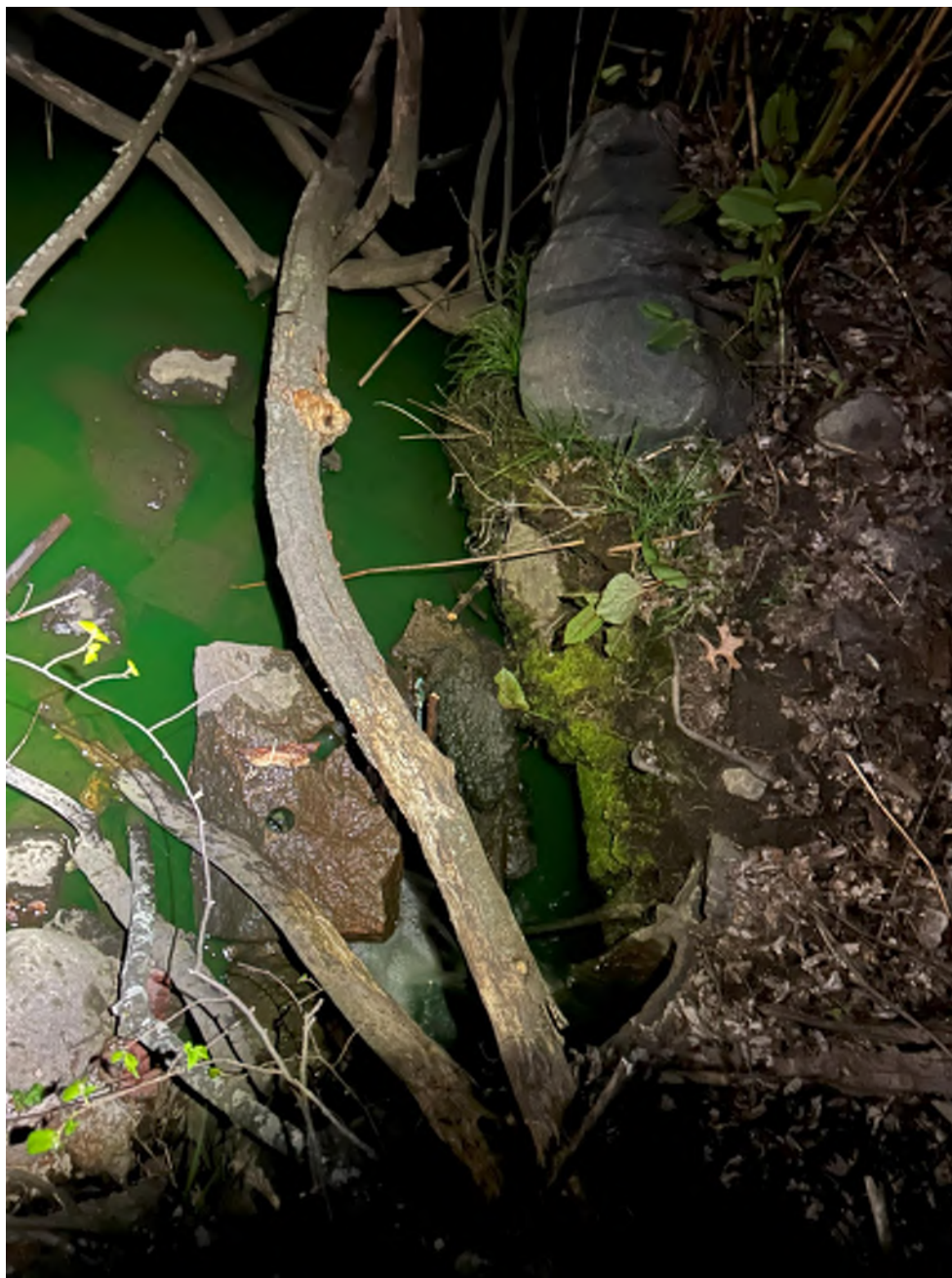
FIGURE 7: FAIRFAX STREET DYE IN ALEWIFE BROOK FROM OUTFALL 11
