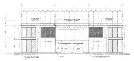
The design change became evident upon final review by Planning Staff and Inspectional Services when the Applicant applied for a Certificate of Occupancy. The three bays of panels are acceptable, but the exposed mechanical louvers create a "rear" appearance to the building that was intended to be a four-sided pavilion. The decorative louvers proposed are an acceptable approach to visually screening the necessary but unsightly louvers.
