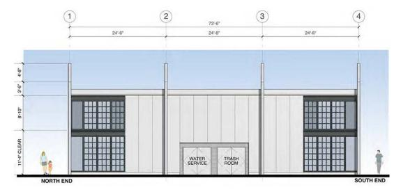
The elevation from the building permit application (shown below) shows reduced fenestration at the north and south ends of the building - three bays instead of four but still showing windows.
