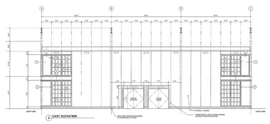
The as-built condition provided with this application (below) shows the extent of the changes that were made during construction without prior Staff or Planning Board approval. Note the mechanical louvers and the blank panels instead of windows.
