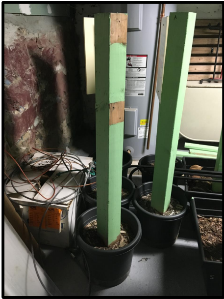
FENCE POSTS & BASES. 4X4 POSTS (3-1/2" X 3-1/2") SECURED WITH SOIL. OVERALL DIMENSIONS: 13" (BASE DIAMETER) 49" (H)
