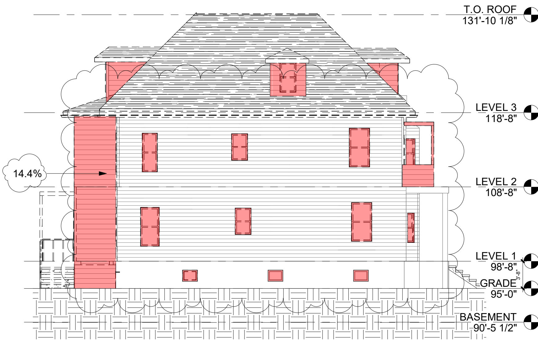
4 EXISTING/ DEMO WEST ELEVATION 1/8" = 1'-0"
