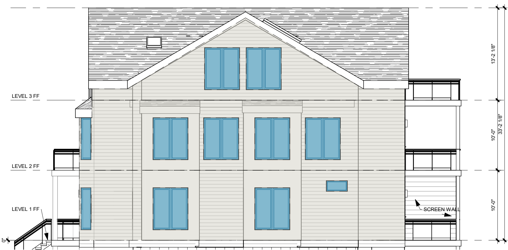
2 FENESTRATION - PROPOSED EAST ELEVATION 1/8" = 1'-0"
