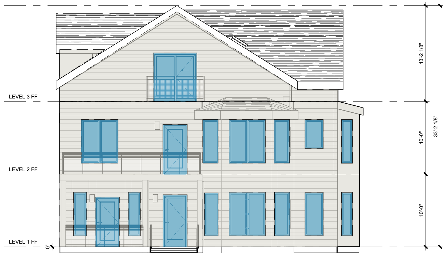
1 FENESTRATION - PROPOSED SOUTH ELEVATION 1/8" = 1'-0"
