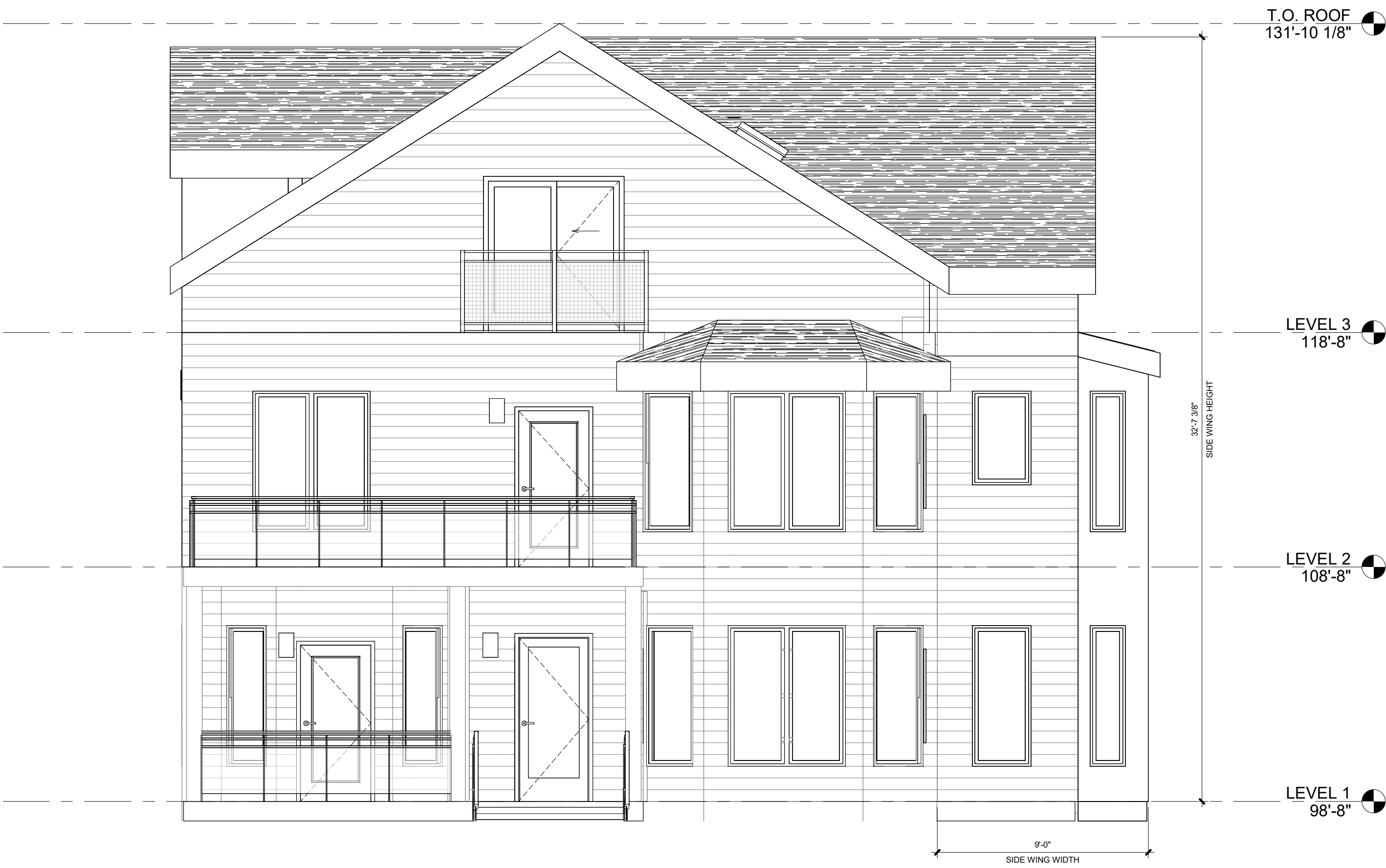
2 SIDE WING - PROPOSED SOUTH ELEVATION 1/4" = 1'-0"
