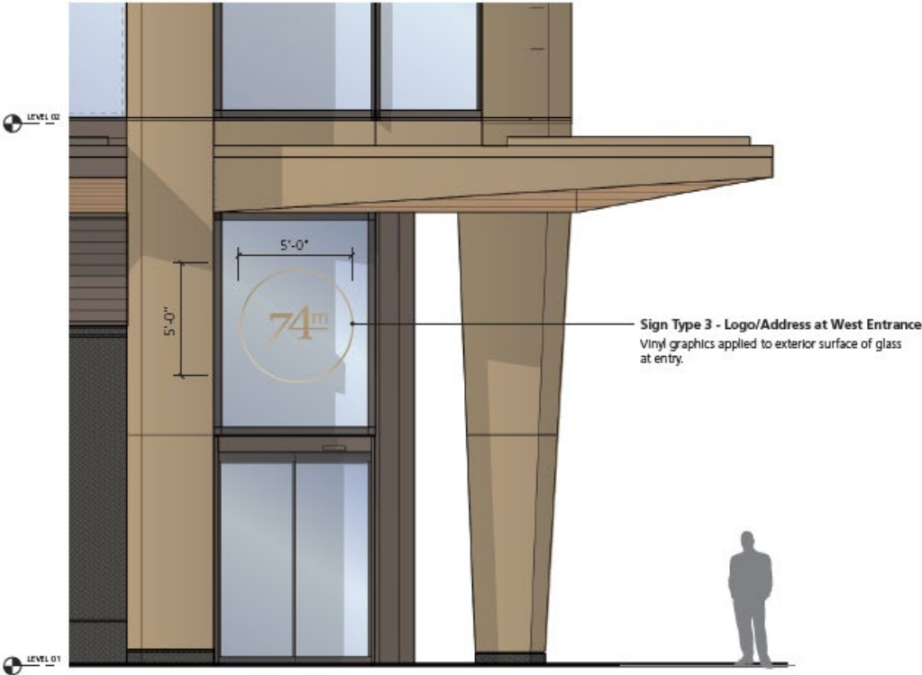
Elevation - West Building Entry Scale: 3/16" = 1' - 0"
