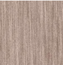
ACRE Wood-like cladding at Entry, made of upcycled rice hulls
