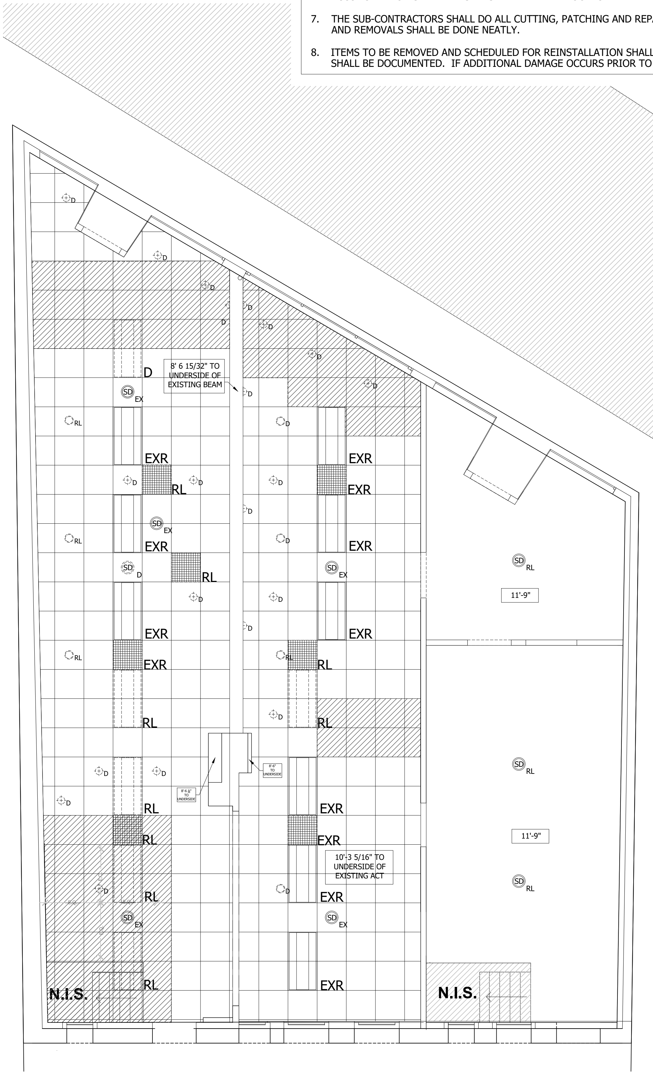
1 GROUND FLOOR DEMOLITION REFLECTED CEILING PLAN 1/4"=1'-0"
