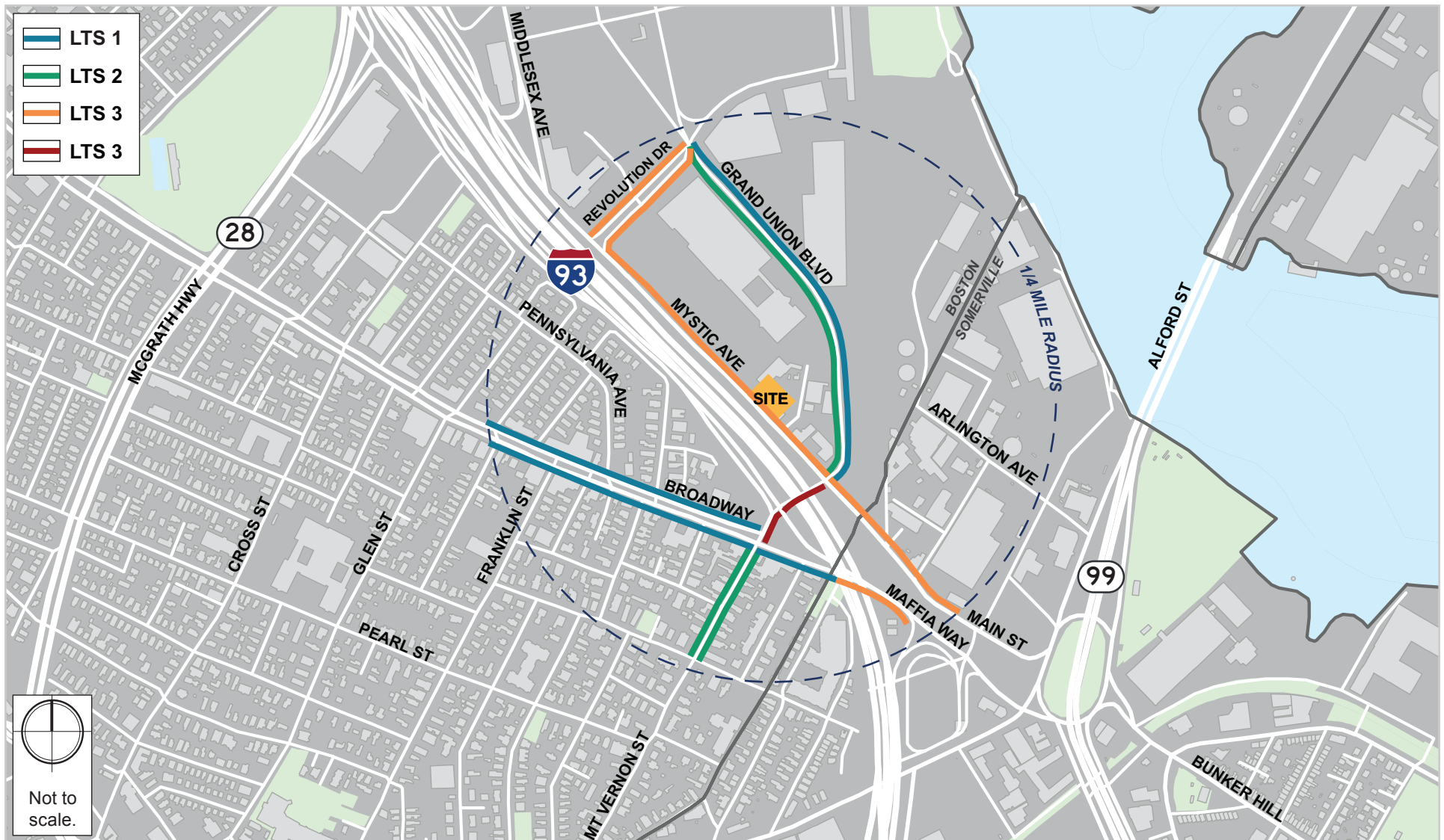
Figure 20. Pedestrian Level of Traffic Stress - Existing
