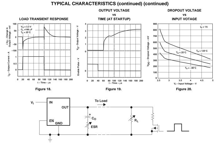
Figure 21. Test Circuit for Typical Regions of Stability (Figure 22 Through Figure 25) (Fixed-Output Options)
