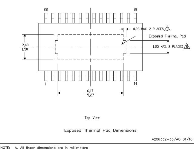
DTE: A. All linear dimensions are in millimeters B. Exposed tie strap features may not be present.
