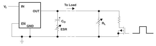
Figure 27. Test Circuit for Typical Regions of Stability (Figure 21 through Figure 24) (Fixed Output Options)
