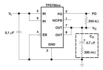
Figure 28. Typical Application Circuit (Fixed Versions)
