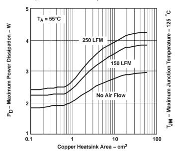
Figure 22. Maximum Power Dissipation vs Copper Heatsink Area
