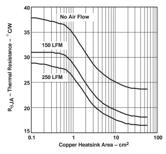
Figure 20. DDPAK Thermal Resistance vs Copper Heatsink Area
