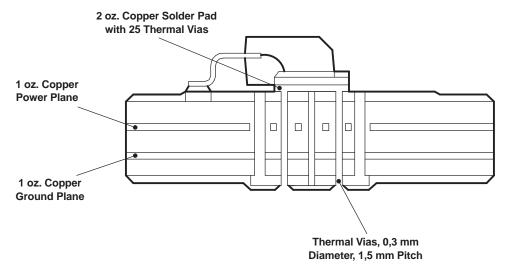
Figure 21. DDPAK Thermal Resistance
