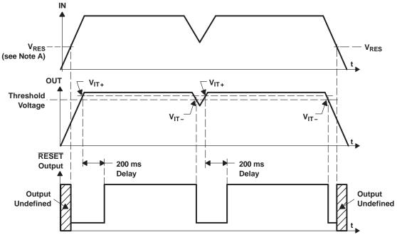
NOTES:A.  $V_{RES}$  is the minimum input voltage for a valid  $\overline{RESET}$ .
