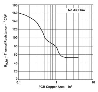
Figure 23. SOT223 Thermal Resistance vs PCB AREA
