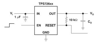
Figure 18. TPS726xx Fixed Output Typical Application Diagram
