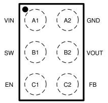
Figure 6-1. YFF Package 6-Pin YFF Top View
