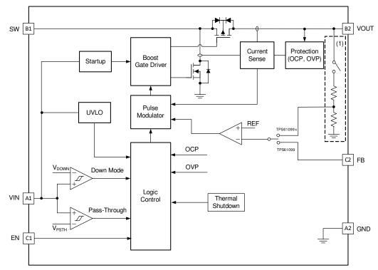
A. Internal FB resistor divider is implemented in fixed output voltage versions.
