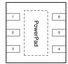
Figure 6-2. DRV Package 6-Pin DRV Top View
