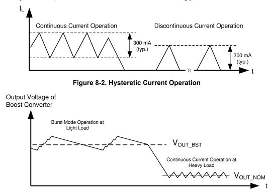
Figure 8-3. Burst Mode Operation
