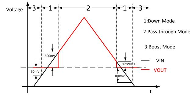
Figure 8-4. Down Mode and Pass-Through Operation
