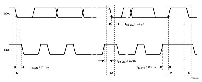
Figure 17. I<sup>2</sup>C Interface Timing
