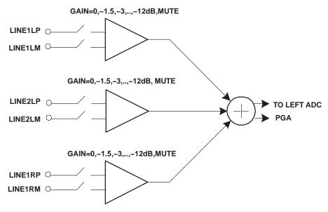
Figure 31. Left Channel Fully-Differential Analog Input Mixing Configuration
