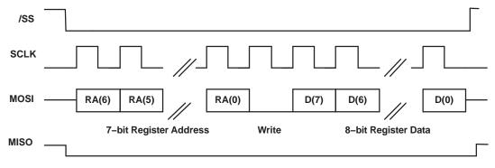
Figure 15. SPI Write
