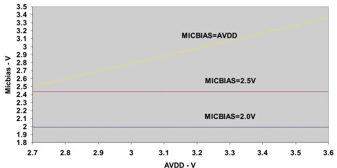
Figure 12. MICBIAS Output Voltage vs AVDD
