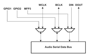
Figure 20. Alternate Audio Bus Mulitplexing Function
