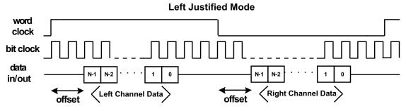
Figure 26. DSP Mode and Left Justified Modes, Showing the Effect of a Programmed Data Word Offset
