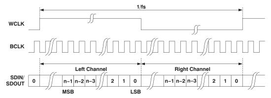
Figure 22. Right Justified Serial Bus Mode Operation
