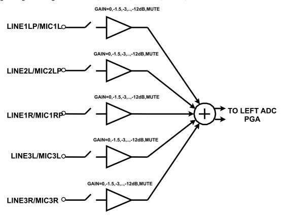
Figure 32. Left Channel Single-Ended Analog Input Mixing Configuration
