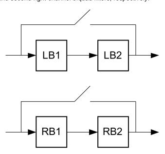
Figure 29. Structure of the Digital Effects Processing for Independent Channel Processing
