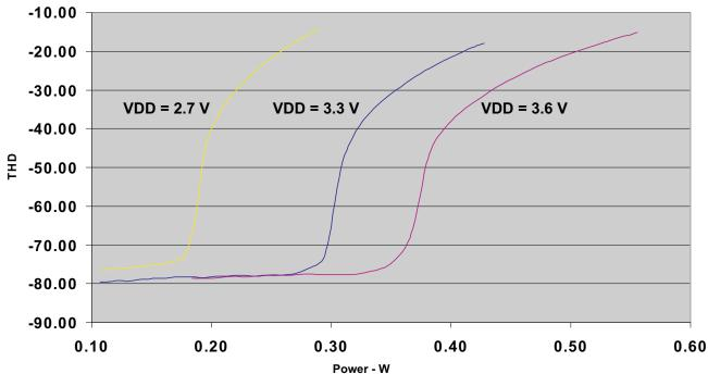
Figure 9. Speaker Power vs THD, 8  $\Omega$  Load
