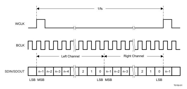
Figure 25. DSP Serial Bus Mode Operation
