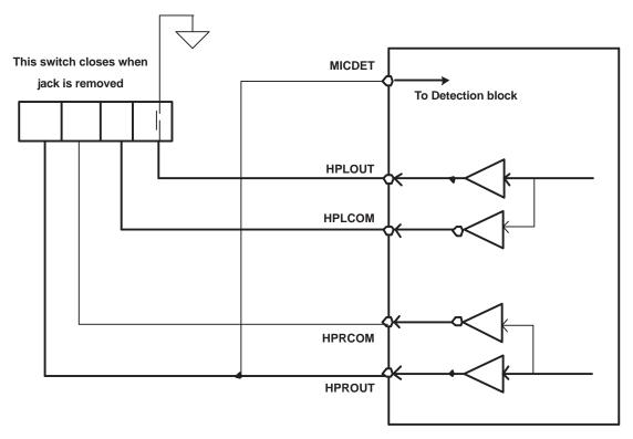
Figure 38. Configuration of device for jack detection using a fully differential stereo headphone output connection.
