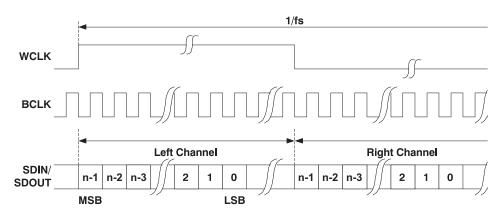
Figure 23. Left Justified Serial Data Bus Mode Operation
