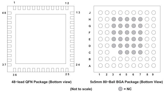
Connect QFN thermal pad to DRVSS.
