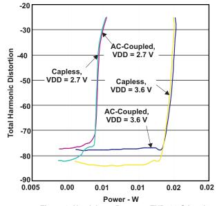
Figure 5. Headphone Power vs THD, 16  $\Omega$  Load Figure 6. Headphone Power vs THD, 32  $\Omega$  Load
