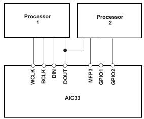
Possible Processor Types: Application Processor, Multimedia Processor, Compressed Audio Decoder, Wireless Modem, Bluetooth Module, Additional Audio/Voice Codec
