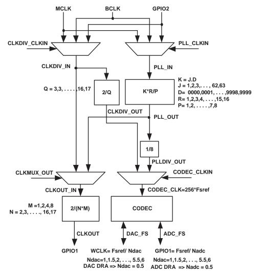
Figure 27. Audio Clock Generation Processing
