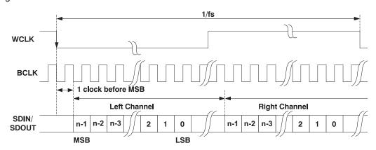
Figure 24. I<sup>2</sup>S Serial Data Bus Mode Operation
