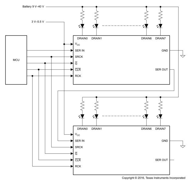
Figure 14. Typical Application Circuit
