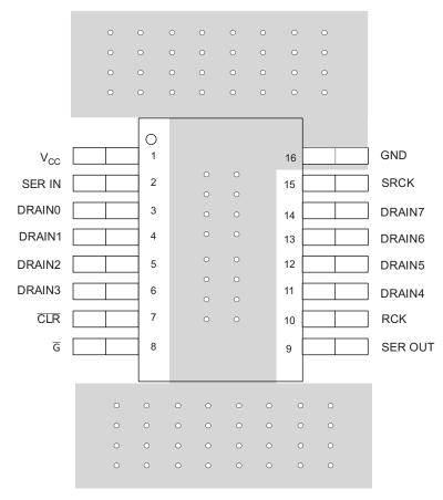
Figure 16. TLC6C598 Example Layout
