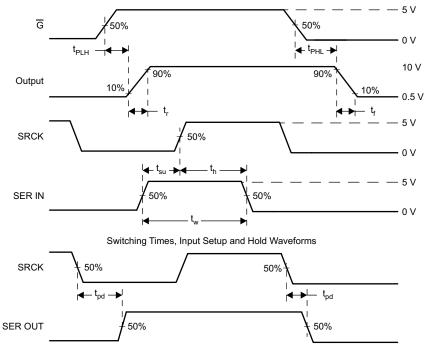
SER OUT Propagation Delay Waveform
