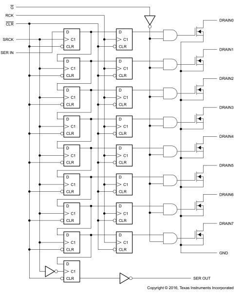
Figure 13. Logic Diagram (Positive) of TLC6C598
