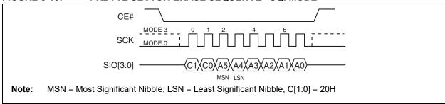
FIGURE 5-20: 4 KBYTE SECTOR-ERASE SEQUENCE (SPI)
