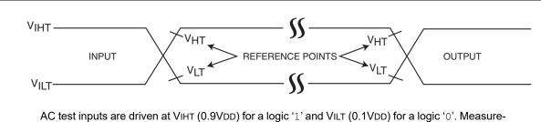
and test inputs are driven at VIHT (0.9VDD) for a logic '1' and VILT (0.1VDD) for a logic '0'. Measurement reference points for inputs and outputs are  $V_{HT}$  (0.6VDD) and  $V_{LT}$  (0.4VDD). Input rise and fall times (10%  $\leftrightarrow$  90%) are <3 ns.
