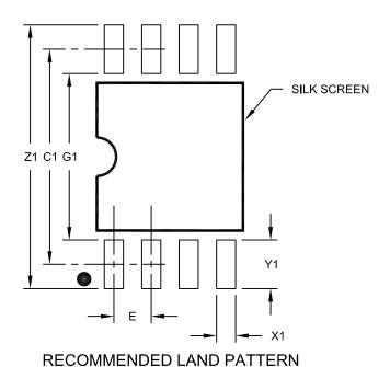
**MILLIMETERS** Units MIN MAX **Dimension Limits** MOM Contact Pitch Ε 1.27 BSC Overall Width Z1 9.00 Contact Pad Spacing C1 7.30 Contact Pad Width (X8) X1 0.65 Contact Pad Length (X8) Υ1 1.70 Distance Between Pads G1 5.60 Distance Between Pads G 0.62
