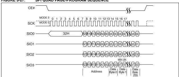
FIGURE 5-27: SPI QUAD PAGE-PROGRAM SEQUENCE
