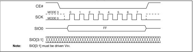
FIGURE 5-5: RESET QUAD I/O SEQUENCE (SQI)
