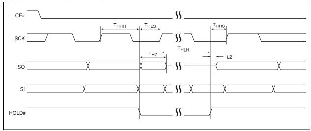
FIGURE 8-2: SERIAL INPUT TIMING DIAGRAM
