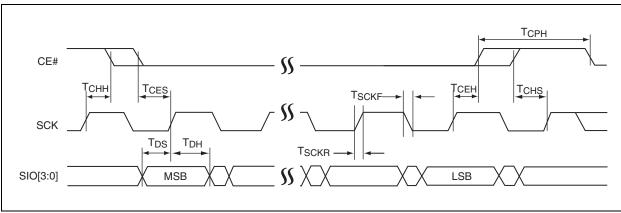
FIGURE 8-3: SERIAL OUTPUT TIMING DIAGRAM
