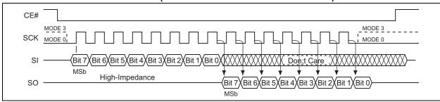
FIGURE 4-2: SQI SERIAL QUAD I/O PROTOCOL
