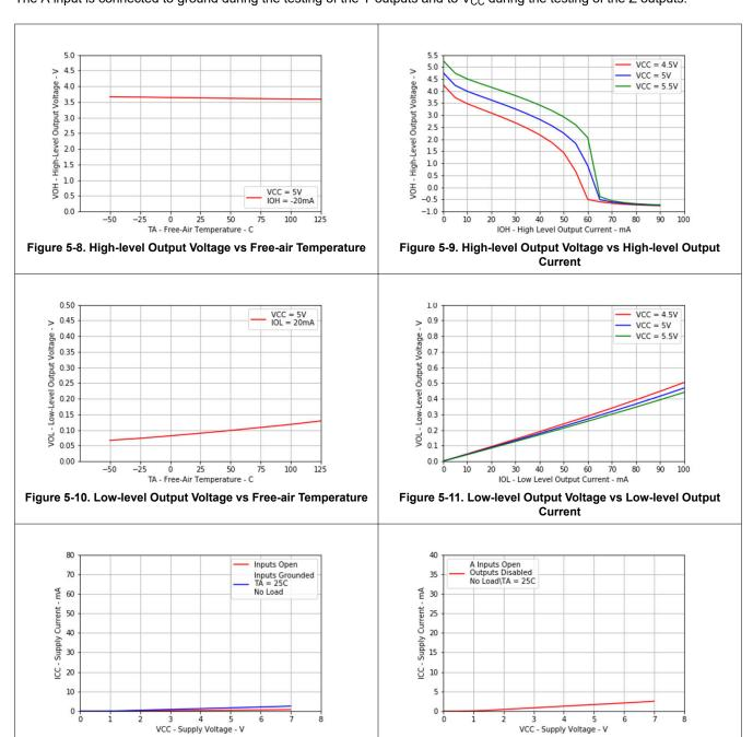
Figure 5-12. Supply Current vs Supply Voltage
