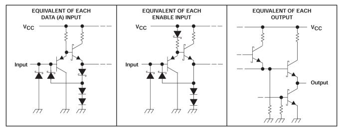
Figure 7-1. Schematics of Inputs and Outputs
