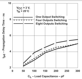
Figure 6-2. Propagation Delay (High to Low Transition)
