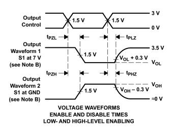
NOTES: A.  $C_L$  includes probe and jig capacitance.
