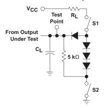
Figure 23. Load Circuit For 3-State Outputs
