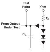
Figure 14. Load Circuit For 2-State Totem-Pole Outputs
