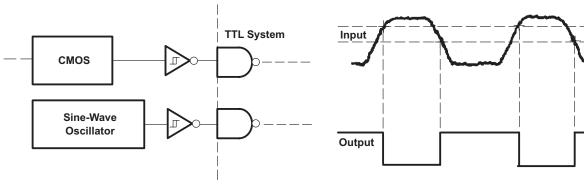
Figure 30. TTL System Interface For Slow Input Waveforms
