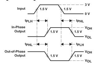
Figure 19. Voltage Waveforms Propagation Delay Times
