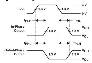
Figure 26. Voltage Waveforms Propagation Delay Times
