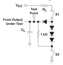
Figure 16. Load Circuit For 3-State Outputs
