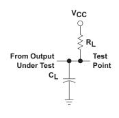
Figure 22. Load Circuit For Open-Collector Outputs
