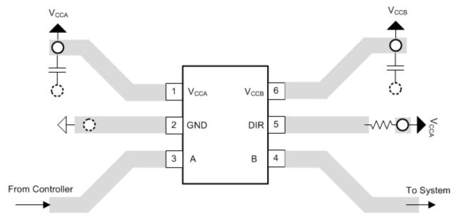
Figure 16. PCB Layout Example
