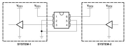
Figure 12. Unidirectional Logic Level-Shifting Application
