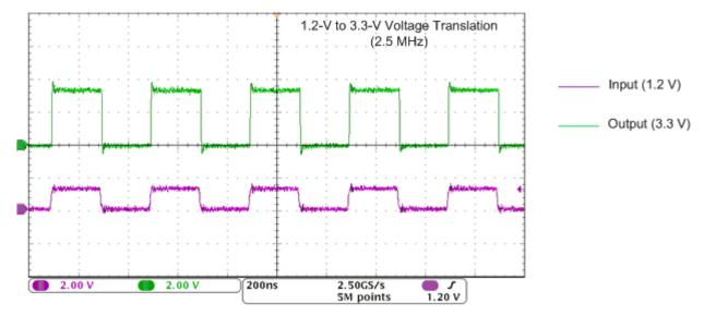
Figure 15. Translation Up (1.2 V to 3.3 V) at 2.5 MHz
