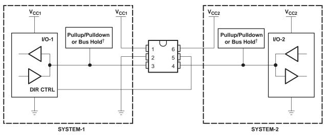
Figure 14. Bidirectional Logic Level-Shifting Application
