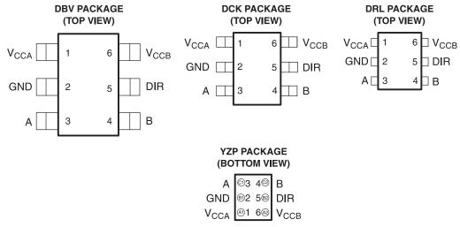
See mechanical drawings in *Mechanical, Packaging, and Orderable Information* for dimensions.
