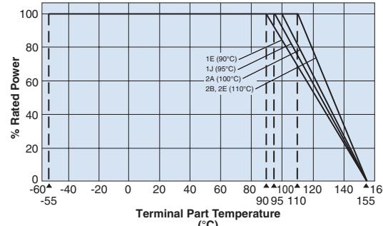
For resistors operated at a terminal part temperature of described for each size or above, a power rating shall be derated in accordance with derating curve. Please refer to "Introduction of the derating curves based on the terminal part temperature" in the beginning of our catalog before use.
