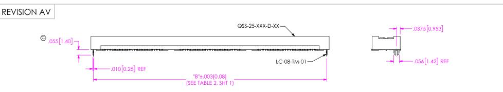
FIG 2 -LC: LOCKING CLIP OPTION (QSS-075-01-XXX-D-LC SHOWN) (DIFFERENT AS SHOWN, OTHERWISE SAME AS FIG 1)
