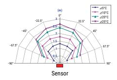
$\Delta T$  (°C) = Difference between room temperature and heat source temperature
