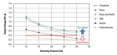
Measuring conditions: Transfer velocity - 1 m/s
