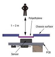
Detecting distance increased to a few meters by using a polyethylene plate.
