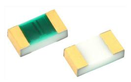
The terminations consist of an adhesion layer, a leach resistant nickel barrier and gold plating compatible with high temperature solder systems.
