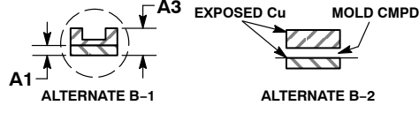
DETAIL B ALTERNATE CONSTRUCTIONS
