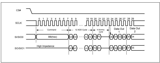
Figure 20. 2 x I/O Read Mode (2READ) Sequence
