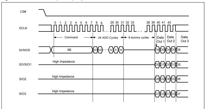
Figure 21. Quad Read Mode (QREAD) Sequence
