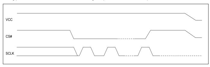
Figure 48. Power-up Timing
