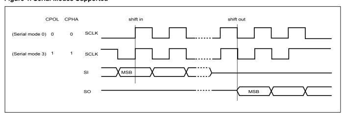
Figure 1. Serial Modes Supported
