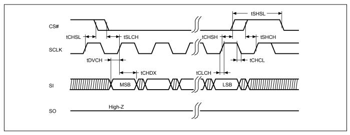
Figure 3. Output Timing
