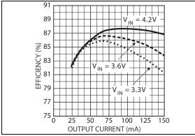
**FIGURE 2-1:** Efficiency at  $V_{OUT} = 12V$ .
