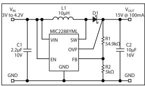
**FIGURE 6-4:** 3.0V to 4.2V V<sub>IN</sub> to 15V<sub>OUT</sub> @ 100 mA.
