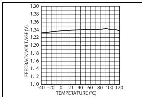
**FIGURE 2-3:** Feedback Voltage vs. Temperature.
