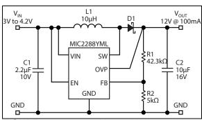
**FIGURE 6-3:** 3.0V to 4.2V V<sub>IN</sub> to 12V<sub>OUT</sub> @ 100 mA.
