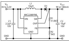
**FIGURE 6-2:** 3.0V to 4.2V V<sub>IN</sub> to 9V<sub>OUT</sub> @ 180 mA.
