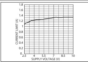
FIGURE 2-4: Current-Limit vs. Supply Voltage.
