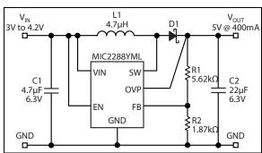
**FIGURE 6-1:** 3.0V to 4.2V V<sub>IN</sub> to 5V<sub>OUT</sub> @ 400 mA.
