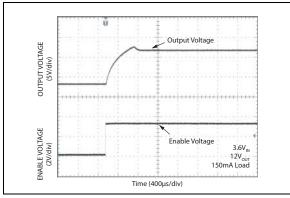
FIGURE 2-13: Enable Characteristics.
