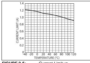
FIGURE 2-5: Current-Limit vs. Temperature.
