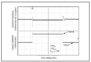
FIGURE 2-15: Load Transient Response.
