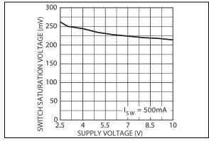
FIGURE 2-6: Switch Saturation vs. Supply Voltage.
